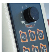
Electronically adjustable speed regulator
